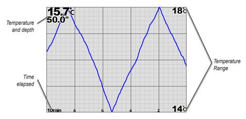
The temperature appears along the right side and the time elapsed appears along the bottom. The graph scrolls to the left as information is received.
